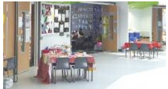
Moveable partitions mean that classrooms can either be opened to linked breakout spaces, or closed off. Courtesy of elder & cannon architects limited.
